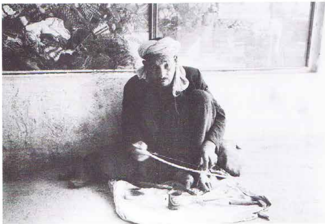
1. Afghani drilling bead with bow drill. (© Irving Mazze. All rights reserved.)
